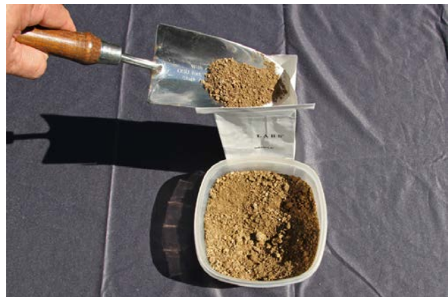
Figure 13: Take about one pint of the composite sample to be sent for testing.
