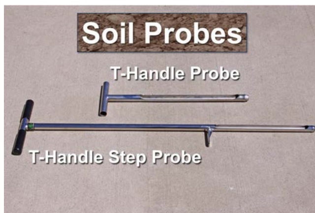
Figure 6: The T-handle probe or T-handle step probe provide a simple method for collecting soil samples. Photo by Joe Boggs, Ohio State University Extension.
